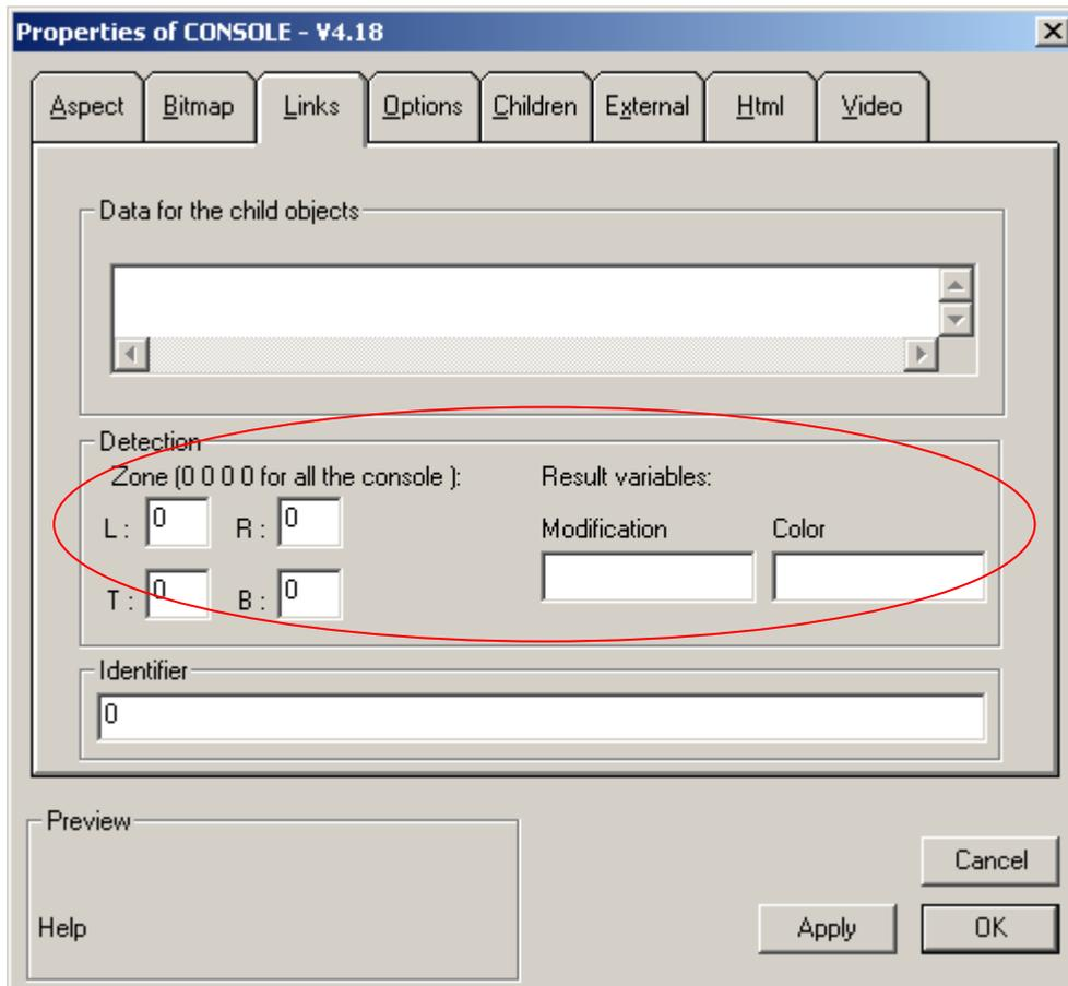
Detection parameters in Link tabulation allow defining detection functions on console window. This is useful with console using a video source for making a moves or color detection. A simple webcam can become a presence sensor or a color sensor.
