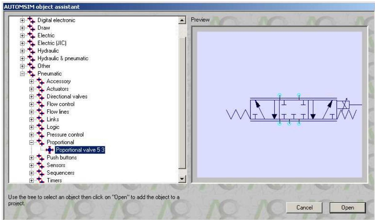
The "Proportional" option can also be checked in any "directional valve" properties.
