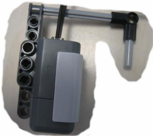
Our light sensor will be arbitrarily wired on input 2 of the brick.
