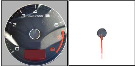
The file used for the moving part (here the right one), must have the same name that the background file with '\_' added at the end of the name. For this sample, gauge6.bmp and gauge6\_.bmp are used. The "white" color is used as transparent for the moving part file.
